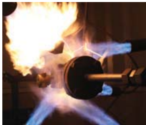
2" 73Z valve in a fire test
